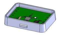
2. Lift electronics board out of assembly and remove battery. Place new battery in same orientation.
